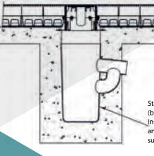
Standard Gully Pot (by others) Installed at depth and orientation to suit invert requirements
